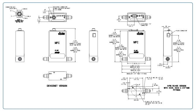
Dimensional Drawing — DeviceNet<sup>™</sup> and RS485 with VCR fittings\* \*(See manual for additional I/O and fitting types) Note: Unless specified, dimensions are nominal values in inches (mm referenced).
